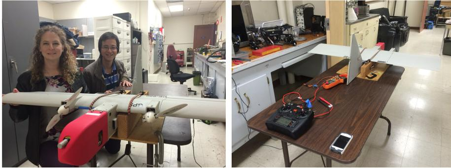
(a) PI Kristin Yvonne Rozier and Ph.D. Research Intern Quoc-Sang Phan assembling a DragonEye on the test stand in December, 2014. (b) DragonEye in a test stand flight test, with motors running, without fan. For tests with a fan, the large fan was placed on a table in front of the test stand.
